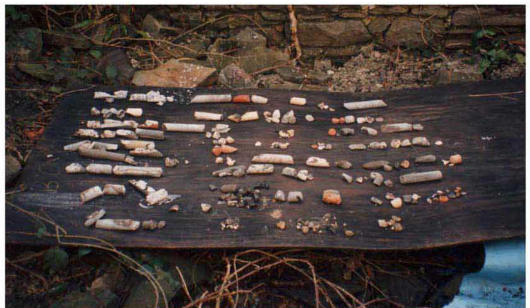
The process of diamond drilling (above), with the subsequent core samples produced, (left).
